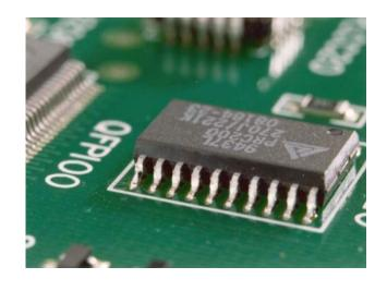
When hand soldering chip components, first clean and tin the soldering bit and place it in contact with the terminations
