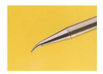
When the soldering iron bit has reached temperature wipe the bit on the moist sponge to remove any of the oxidised solder and flux debris from previous soldering operations
