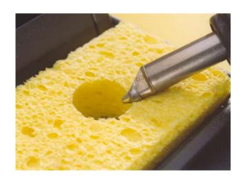
Using the appropriate cored solder wire, tin the de-soldering iron bit prior to desoldering. This will aid heat transfer and speed up the operation. Always re-tin the bit before storing the iron back in the holder
