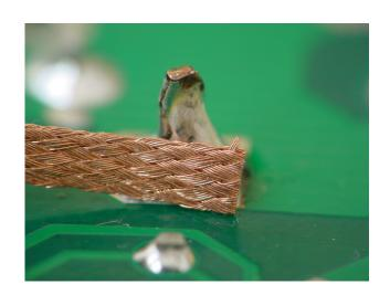
Use a tinned soldering iron tip slightly smaller than the copper braid. Place the tip on the surface, provided the braid is fresh there is no reason to apply any pressure during desoldering
