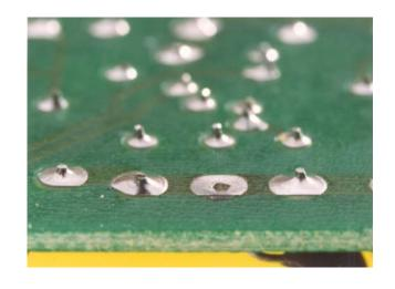
Select a special fine bit soldering iron for the size of termination being soldered and switch the iron on. The bit should be no larger than the termination to be soldered
