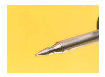
When the soldering iron bit has reached, temperature wipe the bit on the moist sponge to remove any of the oxidised solder and flux debris from previous soldering operations
