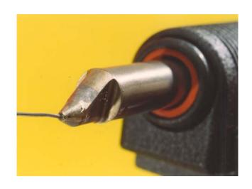
Place the de-soldering iron bit over the lead and wait for reflow of the solder. By rotating the wire termination slightly without pad contact, complete reflow in the plated through hole can be confirmed before applying the vacuum to remove the solder
