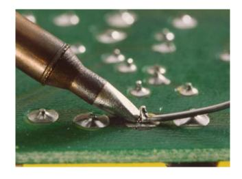
When the joint is completed it should show satisfactory wetting between the termination and the pad surface. If cleaning is required on the product the flux residues around the joint may be removed using a suitable cleaning agent
