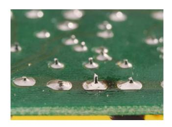
Select the correct de-soldering iron bit for the size of termination being soldered and switch the iron on. The desoldering bit should be slightly smaller than the land; the hole should be slightly larger than the lead diameter
