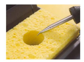
Using the appropriate cored solder wire, tin the soldering iron bit prior to soldering. This will aid heat transfer and speed up the soldering operation. Always re-tin the bit before storing the iron back in the holder
