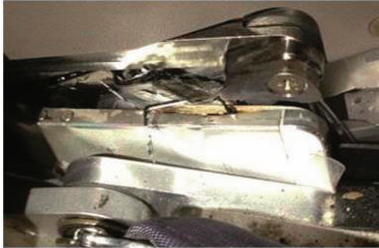
Figure 5.10. A mobile phone crushed in an electrically adjustable seat
