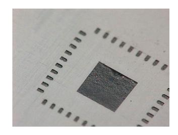
Example of the solder paste deposits on the edge terminations after removal from the stencil and prior to placement. The solder paste aperture on the centre pad is 50-60% of the pad area and printed centrally to reduce displacement of the paste during placement
