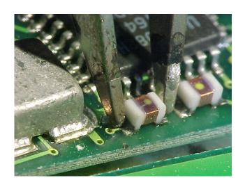
When the solder joints reflow the component can be lifted safely from the surface of the pads
