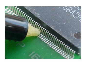
Position the rework head over the device and lower to just above the board surface. Preheat the board assembly using the bottom heater prior to introducing the full heat from the top side and monitor the QFP for reflow
