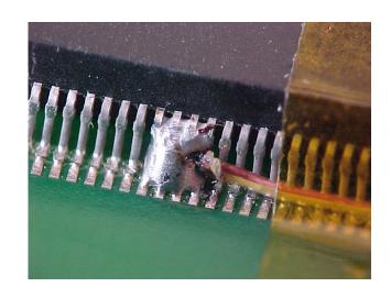
One alternative to high temperature solder for mounting beads is metallised tape which gives a similar performance to soldering the thermocouple beads
