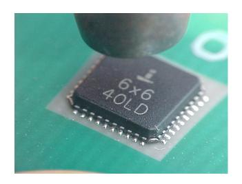
Pads and the centre heat sink may well be an uneven solder coating when the component is removed. If the replacement component cannot be placed parallel on the surface of the board the solder must be levelled
