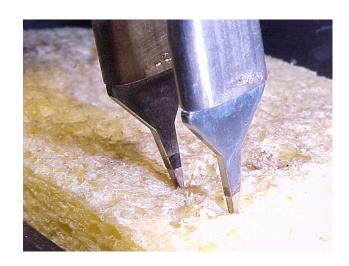
After cleaning, tin the surfaces of the tips with cored wire which will contact the component terminations. The tinning operation will speed up heat transfer for reflow of joints or protect tips when not being used
