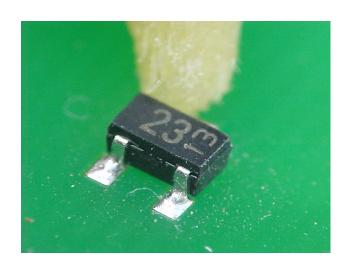
Using a hot air pencil reflow the solder joints, avoid using too higher air pressure so that components are not blown off the pads. The flux on the surface of the joint makes it easier to see reflow of the joints taking place
