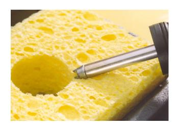
After cleaning tin the surfaces of the tip which will contact the component lead terminations. The tinning operation will speed up heat transfer for reflow of joints
