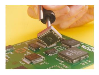
On large pad surfaces with multi pin devices it is often necessary to remove excess solder from the surface of the pads. Solder wick can be used with a long wedge blade to level the pads, care must be taken not to apply pressure to the pads and damage the board
