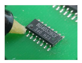
Using a hot air pencil reflow the solder joints, move the hot air pencil over the leads to even out the heating. The flux on the surface of the joint makes it easier to see reflow of the joints taking place
