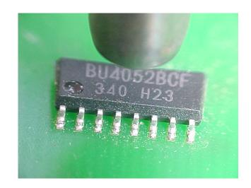
When the solder reflows on both joints lift the component off the surface of the board using a pair of fine tip tweezers. If you are not sure complete reflow has taken place just touch the body lightly to detect complete reflow. Check the surface of the pads for any damage
