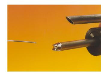
Place the tinned tip in contact with the component terminations and watch for reflow of all terminations. When reflow is complete lift the tip off the surface of the joints. Surface tension of the solder should also lift the component from the pad surface
