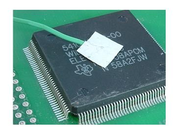
Comparing the component body, printed circuit board and solder joint temperature is normal practice during rework. Try to avoid too much solder being used when checking the solder junction
