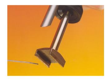
Place the tinned tip in contact with the component terminations and watch for reflow of all terminations. When reflow is complete lift the component from the pad surface. Large components may also require a pair of tweezers to be used
