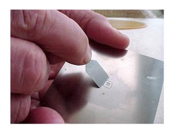
After printing inspect all solder paste apertures for complete fill. After satisfactory printing the stencil can be placed on a rework station and the component lifted directly from the stencil.
