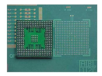
Select a thermocouple lead and place on the surface of the board. Hold the lead in position with Kapton tape. The bead is positioned on the centre pads. Solder the bead to a group of four pads with high temperature solder
