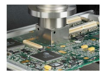
When all the terminations are reflowed the package can be lifted from the board surface using the vacuum pick-up on the machine. Alternatively a manual vacuum tool may be used
