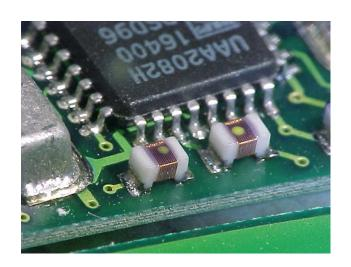
Place the tinned tips of the heated tweezers to contact the component terminations and wait till complete reflow has taken place. There is no need to apply pressure as the tinned tips will allow reflow to take place
