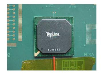
After initial reflow, place adhesive around the four sides of the component and cure the adhesive. This will reduce the possibility of the component coming off the board even when reflowed upside down
