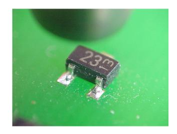
When the solder reflows on both joints lift the component off the surface of the board using a pair of fine tip tweezers. Check the surface of the pads for any damage
