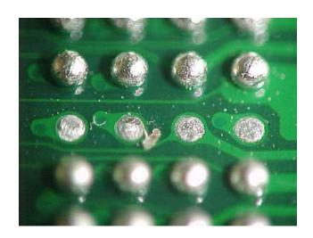
Place the BGA on to the surface of the board making sure that it sits flat on the pads. If the component does not sit flat then remove it. Reposition the lead, flux the pads and replace the BGA
