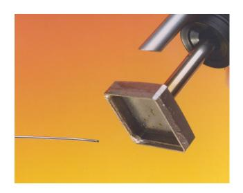
When the tip is in contact with the terminations wait till complete reflow has taken place. At that point the component can be lifted from the surface of the board. Care needs to be taken that all terminations have reflowed on the board and the component does not fall out of the special tool
