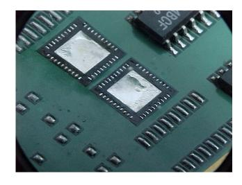
Solder wick may be used to remove the excess solder on the centre pad. If required a smaller gauge of wick is used for the component pads
