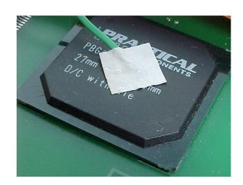
Both quad flat packs and area array devices will have a maximum temperature range for soldering specified by the supplier. Metallised tape can be used to cover the bead of the thermocouple to monitor the temperature rise
