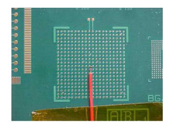
Hold the component firmly and locate the row of balls leading to the centre position of the component
