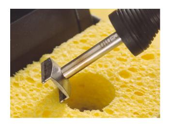
After cleaning, tin the surfaces of the tip that will contact the component terminations. The tinning operation will speed up heat transfer for reflow of joints and aid component removal
