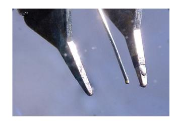
If tinning of the tips is found to be difficult a tip cleaning paste may occasionally be used. Touch the tips on the surface of the paste, do not rub or push the tips deep in to the paste. Check that tip tinning has been successful
