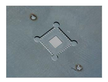
When the component has been placed in position in the stencil cavity there should be limited movement of the component to prevent misalignment of the paste on the terminations
