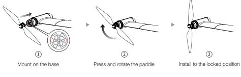
$\square \longrightarrow$  Locking direction: Press and Rotate in the indicated direction to lock the propeller.
