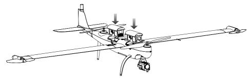
• Align the battery to the battery interface on the fuselage and install it.
